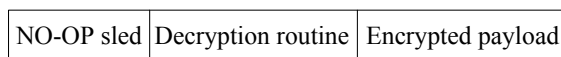
Figure 1.2: A typical structure of a polymorphic exploit of a buffer overflow vulnerability.
